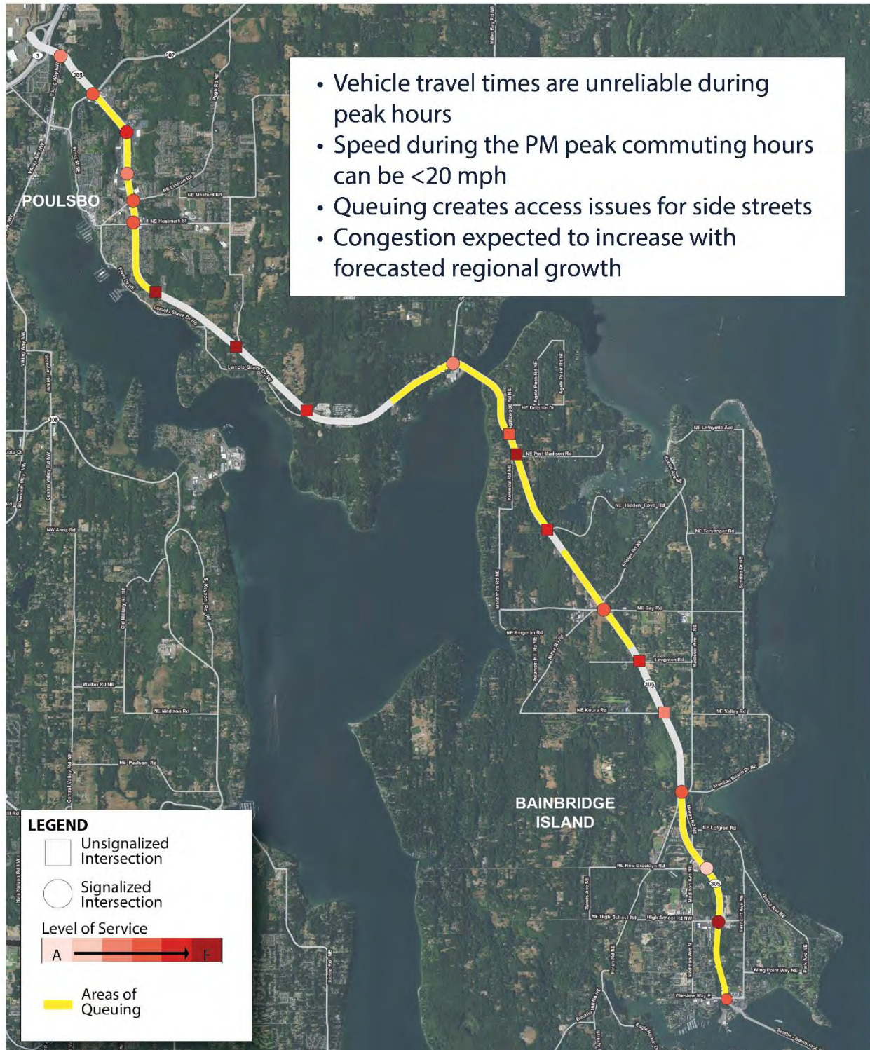
Figure 8. Existing Level of Service and Queues
