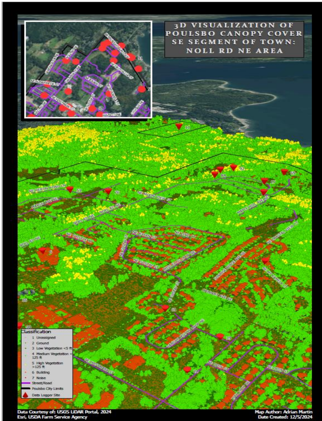
Figure 18: The above figure represents a 3D LiDAR visualization of the variable structured forests, canopy cover, and canopy height in Poulsbo’s Southeast segment. Canopy height varied from <5ft to >125ft. The red indicates buildings while the bright green represents vegetation less than 125ft. The yellow represents vegetation above 125ft.
