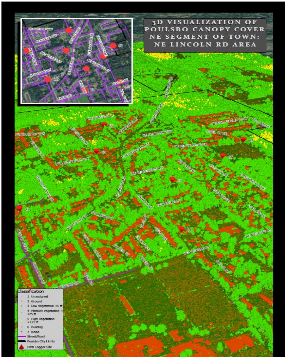
Figure 22: The above figure represents a 3D LiDAR visualization of the variable structured forests, canopy cover, and canopy height in Poulsbo's Northeast segment. Canopy height varied from <5ft to >125ft. The red indicates buildings while the bright green represents vegetation less than 125ft. The yellow represents vegetation above 125ft.
