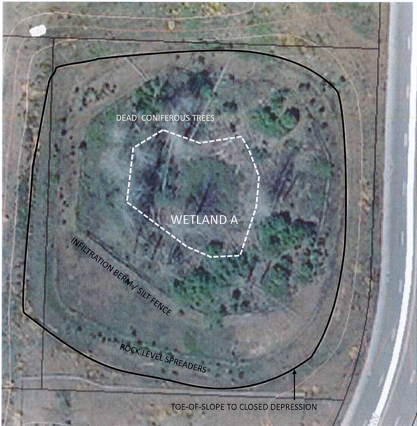
EXHIBIT C: OBSERVED CONDITIONS OF CLOSED DEPRESSION
